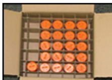
CORRECT (Protective caps in place)
